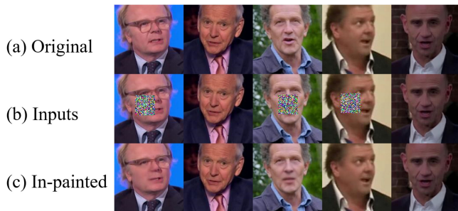
Fig. 10. Examples of (a) original video snapshots; (b) randomly occluded video; and (c) restored video obtained using the in-painting network.
